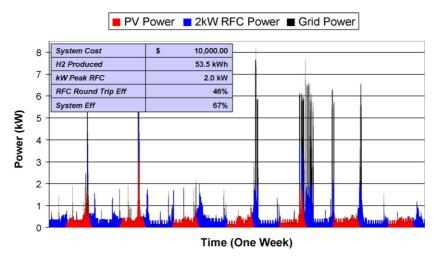
Fig. 8. Residential electrical load demand met by 6 kW photovoltaic array, the grid, 2 kW fuel cell and 7.3 kW electrolyzer with power density limits.
