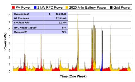
Fig. 9. Residential electrical load demand met by 6 kW photovoltaic array, the grid, 2820 Ah battery, 2 kW fuel cell and 7.3 kW electrolyzer with power density limits. Control strategy uses battery before fuel cell.
