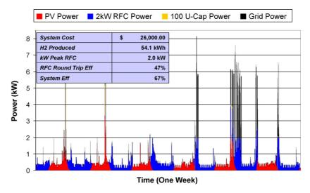
Fig. 11. Residential electrical load demand met by 6 kW photovoltaic array, the grid, 100 ultra-capacitors, 2 kW fuel cell and 7.3 kW electrolyzer with power density limits. Control strategy uses fuel cell before ultra-capacitor.
