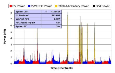
Fig. 10. Residential electrical load demand met by 6 kW photovoltaic array, the grid, 2820 Ah battery, 2 kW fuel cell and 7.3 kW electrolyzer with power density limits. Control strategy uses fuel cell before battery.
