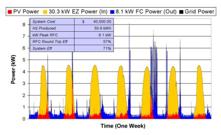
Fig. 5. Supply and demand power flow for a 6 kW photovoltaic array, an 8.1 kW fuel cell, and a 30.3 kW electrolyzer plotted over 1 week.
