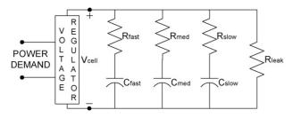
Fig. 2. R-C model of an ultra-capacitor system.
